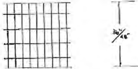
FIGURE 2-59 - VINYL COATED WELDED WIRE CONTAINMENT FENCING
