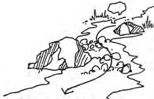
Use of natural materials in man-made drainage channel.
